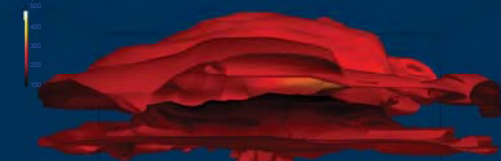
Isosurface of mass concentration m=0.2 of the finest particles. Color scale represents particle temperature.
