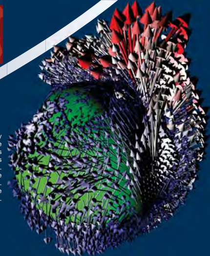
Vector plot of the velocity fluctuations over the interface of the droplet (in green); high turbulence regions are shown in red, whereas low turbulence regions are shown in blue.
